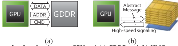
Figure 3. Interface between GPU and (a) GDDR and (b) HMC memory devices.
