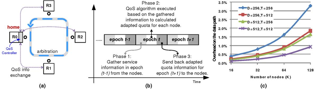
Figure 3: FeatherWeight scheme. (a) optical arbitration hardware for the data channels of R0, (b) timing diagram for an epoch, (c) bandwidth overhead for  $D$ -bit datapath and epoch size of  $T$ .
