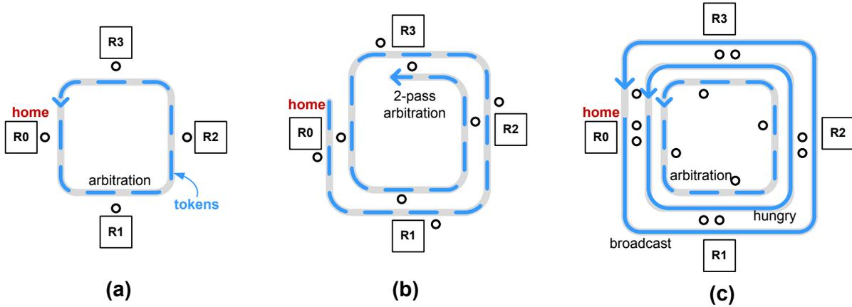
Figure 2: Hardware for (a) baseline optical arbitration, (b) 2-pass Token Stream, and (c) Fair Slot. Waveguides carrying laser (e.g., optical tokens) traverse all the routers for information delivery.
