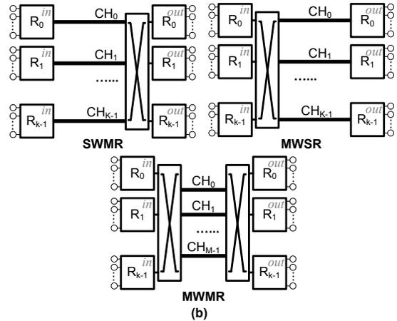
Figure 1: (a) Nanophotonic components and (b) logical architecture of optical crossbars [26].
