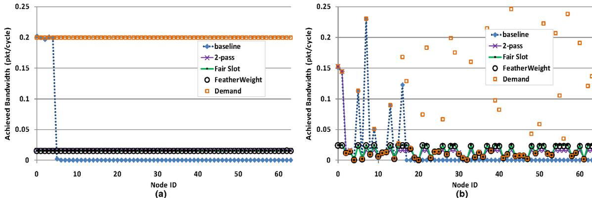
Figure 5: Achieved bandwidth per-node on the channel dedicated to Node 0. (a) equal demand of  $0.2$  pkt/cycle (b) random demand. Demand levels of each node are indicated by the squares.
