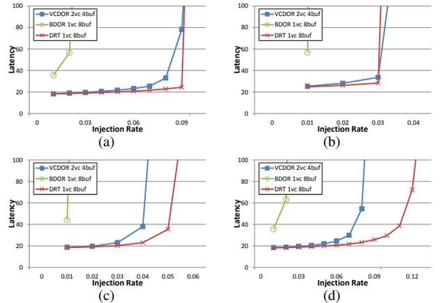
Fig. 7. Comparison for (a) uniform random, (b) tornado, (c) bit reversal, and (d) bit complement traffic pattern in the 8x8 torus network with 8 buffer and 4-flit packets. Injection rate is measured in packets per cycle for each node.
