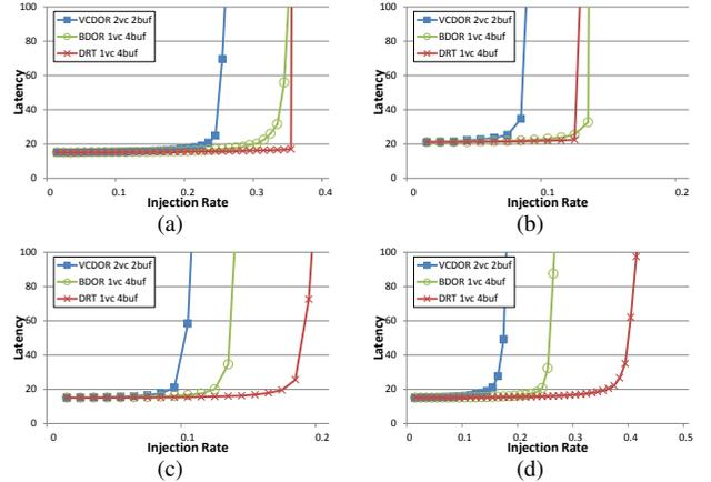
Fig. 6. Comparison for (a) uniform random, (b) tornado, (c) bit reversal, and (d) bit complement traffic pattern in the 8x8 torus network with 4 buffer and 1-flit packets.
