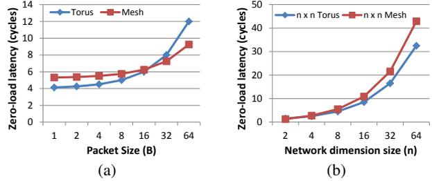
Fig. 2. Zero-load latency comparison of a mesh and a torus (a) as packet size is varied in a  $8\times 8$  network and (b) as network size is increased.
