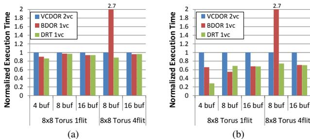
Fig. 8. Closed loop simulation results for (a) uniform random and (b) bit complement traffic pattern.
