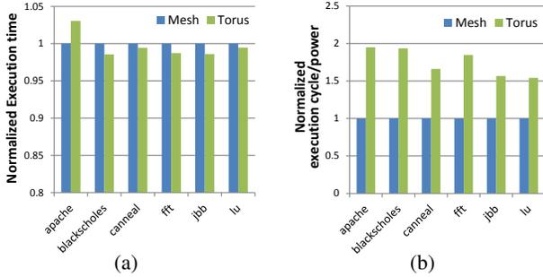
Fig. 1. (a) Performance and (b) performance/watt comparison between a torus and a mesh network. Mesh topology has 16B channel while the torus has 8B channels. Note the zoomed in y-axis for (a).
