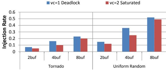
Fig. 3. Network injection rate when the network is saturated ( $vc = 2$  data) and the lowest injection rate when first routing deadlock is detected ( $vc = 1$  data).
