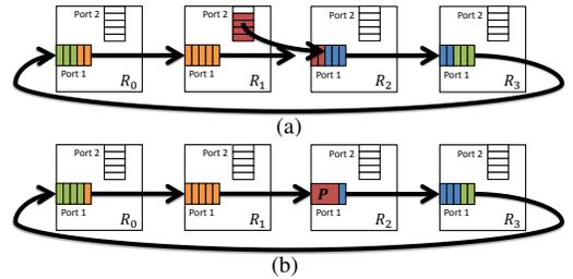
Fig. 4. Routing deadlock scenarios in a 1D torus. Different color represents different packets.
