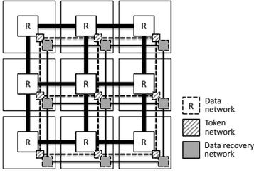
Fig. 5. Network architecture with three parallel networks including the data network, token network, and deadlock recovery network.
